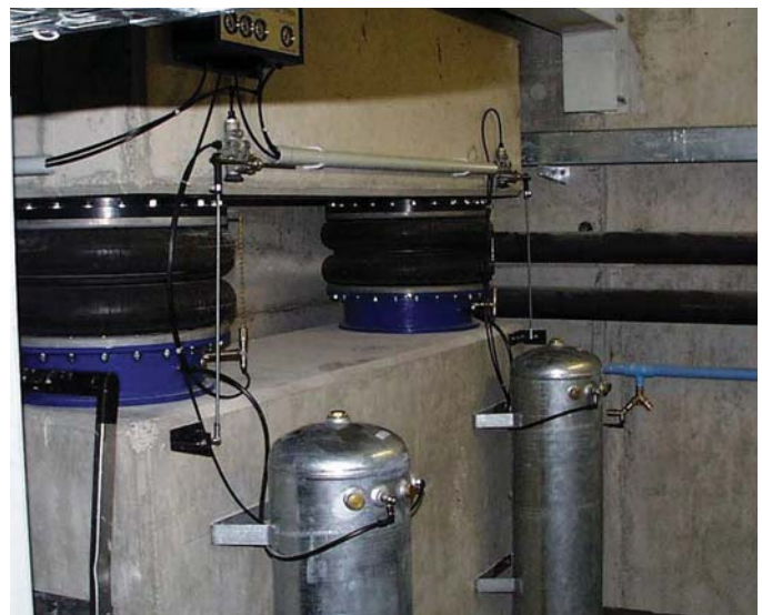
Double convolution air bags designed with additional air volume (auxiliary tanks), damping chambers and leveling valves. This isolation system supports a reaction mass with a bedplate for an engine/dynamometer test rig.
