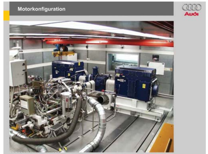
Engine/dynamometer testing on bedplate and support foundation.
