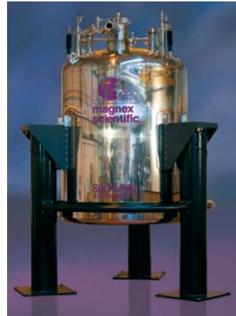
Above left, 800 MHz magnet supported on three PAL133-72P isolators (Photo courtesy of Magnex Scientific)
