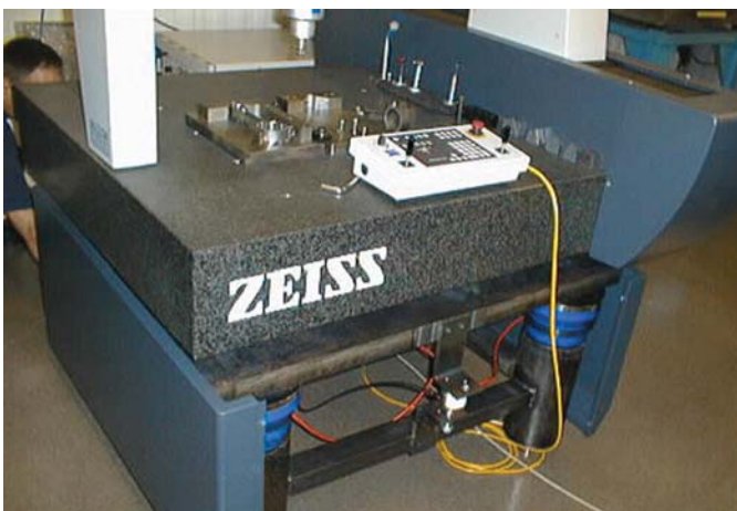
PAL isolators integrated into a coordinate measuring machine support frame.
