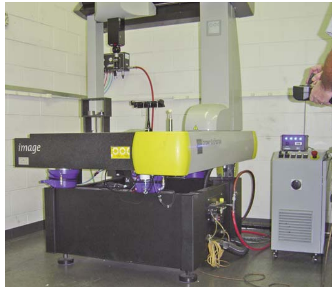
Delta K pneumatic isolation system module allows the Brown & Sharpe Global 7.10.7 CMM to operate at its designed speed and accuracy when supported on pneumatic isolators.
