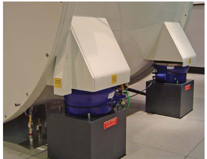
Varian horizontal cryostat (Photo courtesy of Astra-Zeneca)
