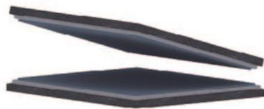
GGX Expansion Bearings are used when temperature is a factor in excess of 275°F. The GGX Expansion Bearings achieve effective performance in environments where temperatures range from -50°F to 700°F. Maximum compressive design stress is 2,000 PSI (14N/mm<sup>2</sup>). The minimum thickness of carbon steel and graphite is 1/4".
