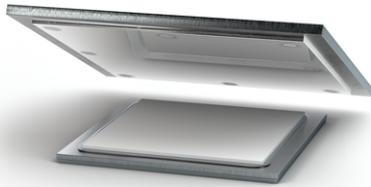
STX Expansion Bearings are used when construction tolerances and loads are moderate. This bearing has an extremely low coefficient of friction, which is exceptional for use where expansion is large. Maximum compressive design stress is 2,000 PSI (14N/mm<sup>2</sup>).
